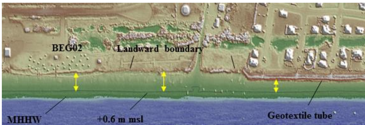
Figure 12. Lidar topographic-relief image of Galveston Island State Park and Pirates Beach subdivision. Note the difference in beach width between the natural beach and the area in front of the subdivision. From Gibeaut and others (2003).
