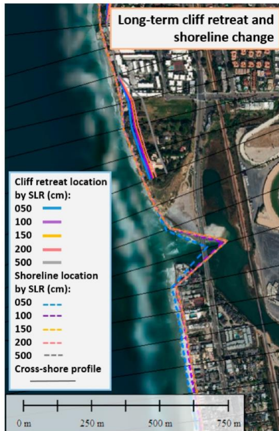
Figure 3.12 CoSMoS simulation results for long-term projected cliff retreat and sandy beach shoreline change under various sea level rise scenarios at seaward lagoon entrance of Del Mar, California [84].
