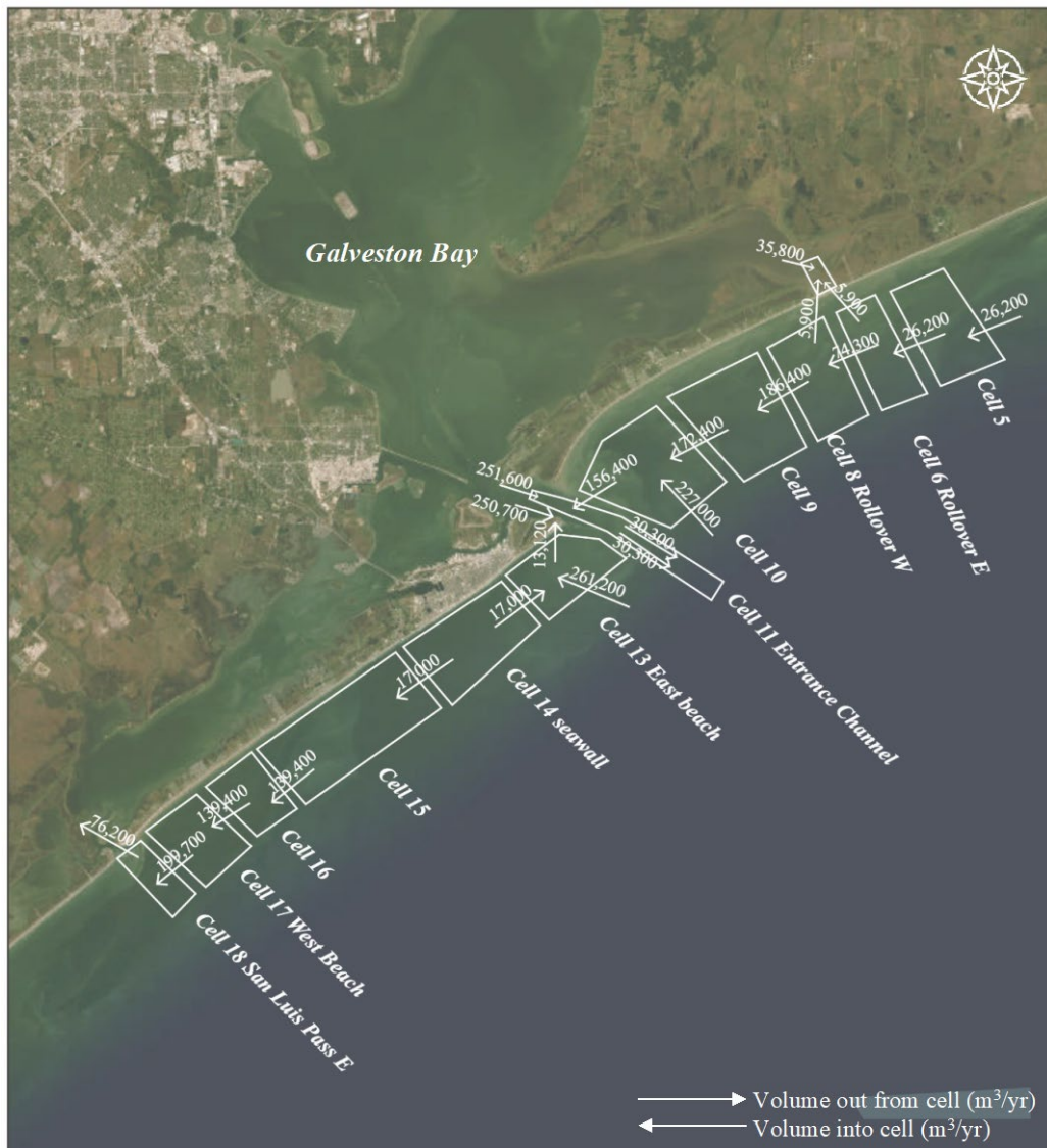
Figure 3.11 Galveston Bay Sediment Budget (Reproduced from Ref. [25])
