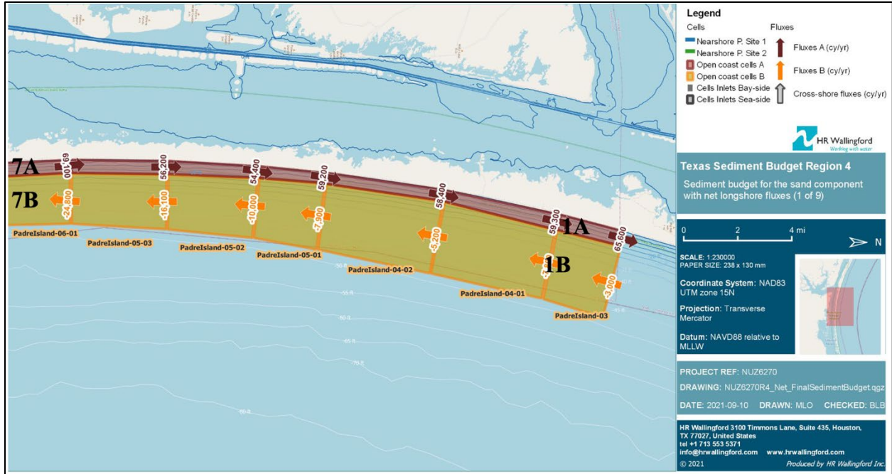
Figure 3.44 Sediment Budget of Laguna Madre System (Cells 1 to 7) in Ref. [177]
