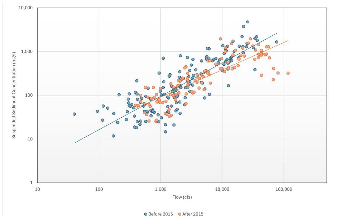
Figure 13 Nonstationary of sediment rating curve at Rosharon Station can be seen by separating the data collected before and after 2015
