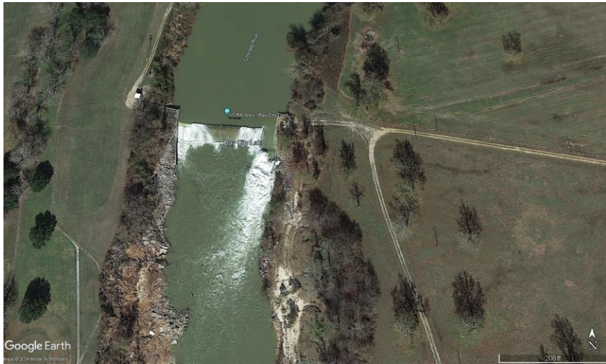
Figure 27 Examples of different hydraulic conditions resulting from the existing spillway structure at the Lower Colorado River Authority's Bay City Dam
