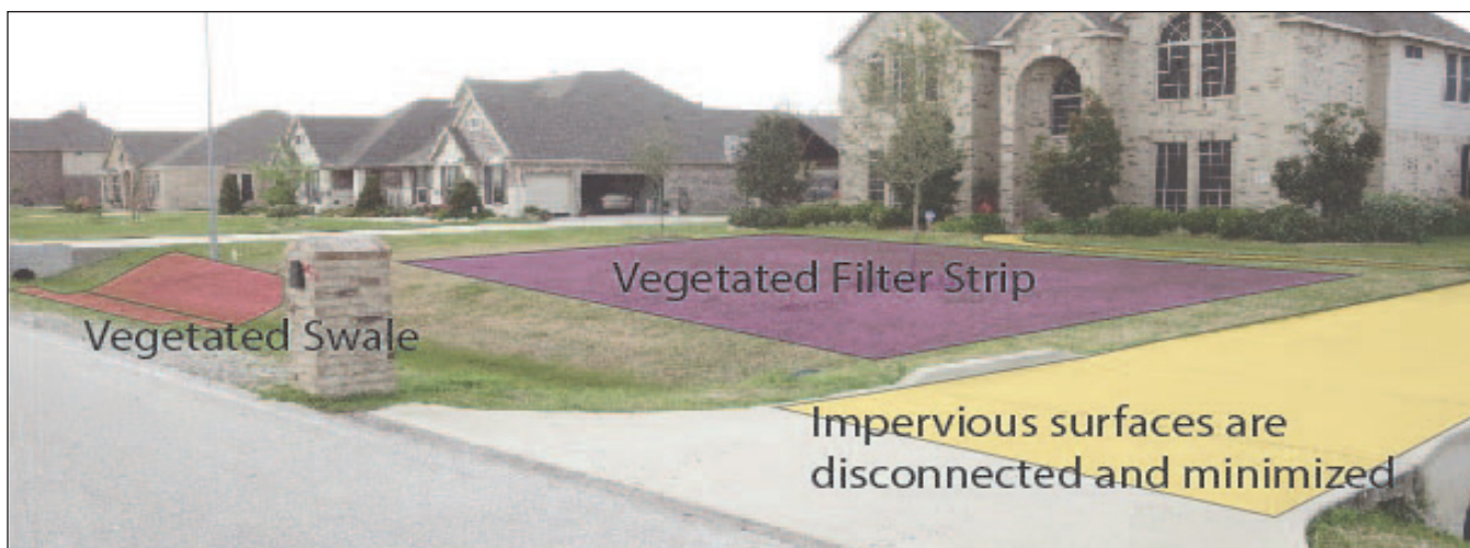
Figure 5-5: Medium density neighborhood uses vegetated swales for stormwater conveyance. These swales also provide water quality benefits.
