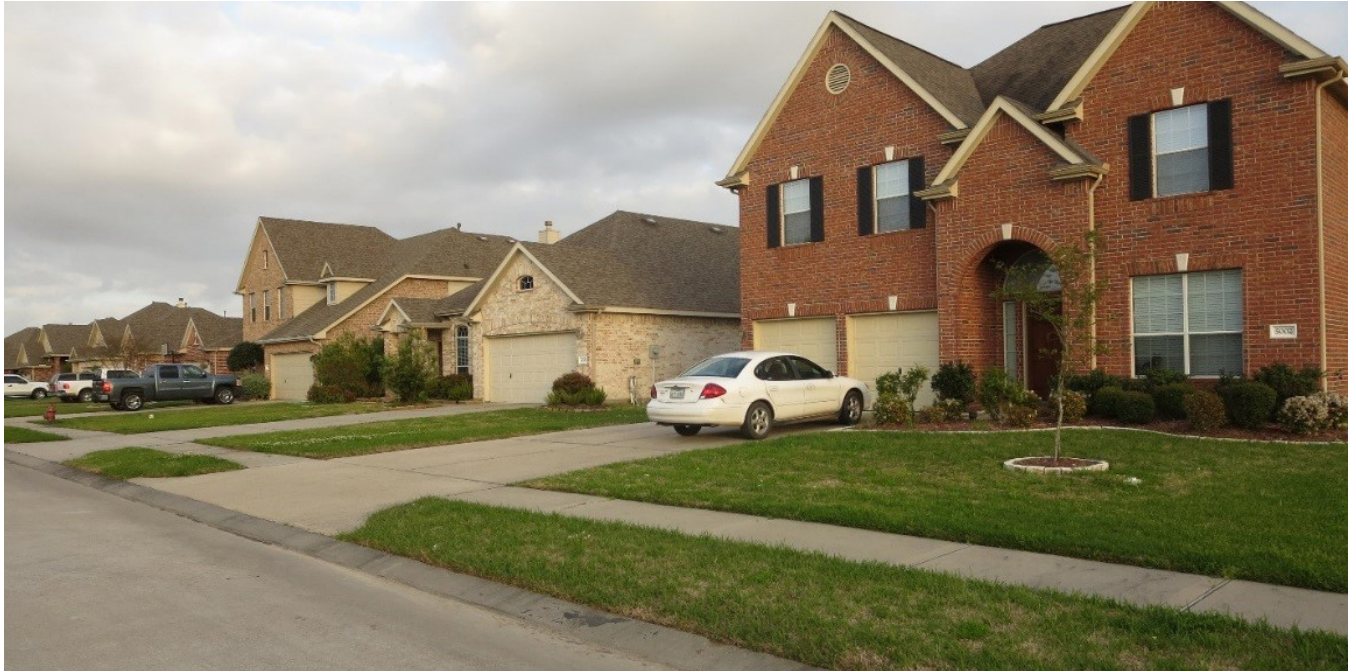
Figure 5-6: Disconnected and minimized impervious cover in Chambers County, Texas.
