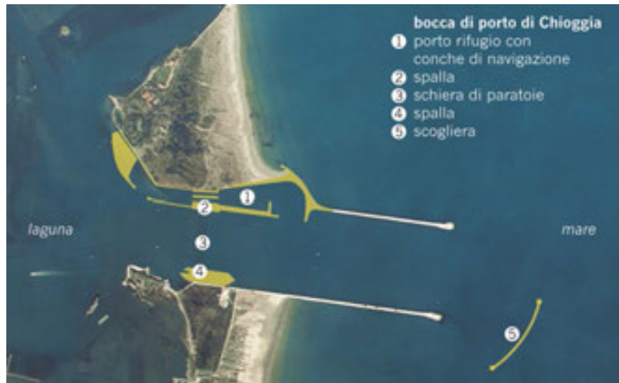
Figure 52 - Chioggia Inlet Barrier
