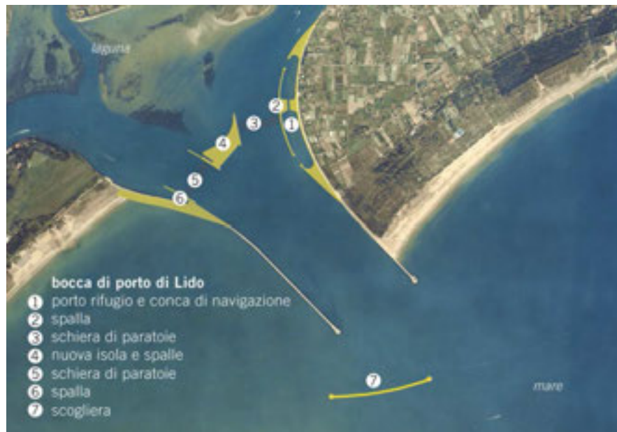
Figure 50 - Lido Inlet Barrier
