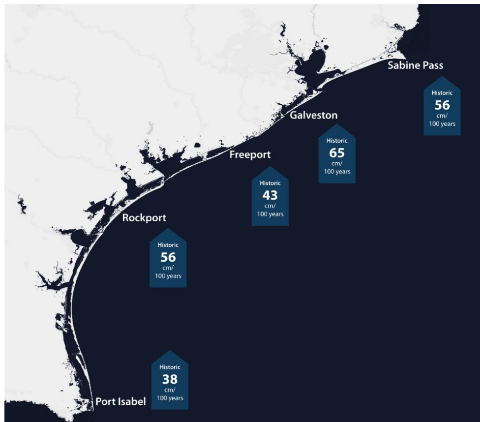
Figure 6-3. Historic RSLR rates on the Texas coast measured by tide gauges
