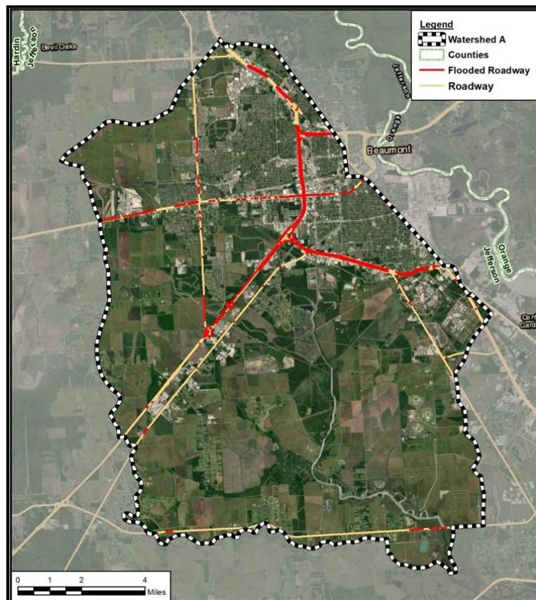
Figure 6. Example Watershed A Flooded Roadways for 1% AEP
