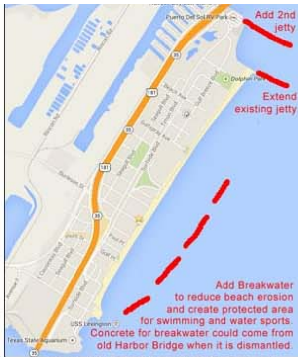
Proposed North Beach Breakwater, aimed at providing a long-term solution to beach erosion. (Click to enlarge map)
