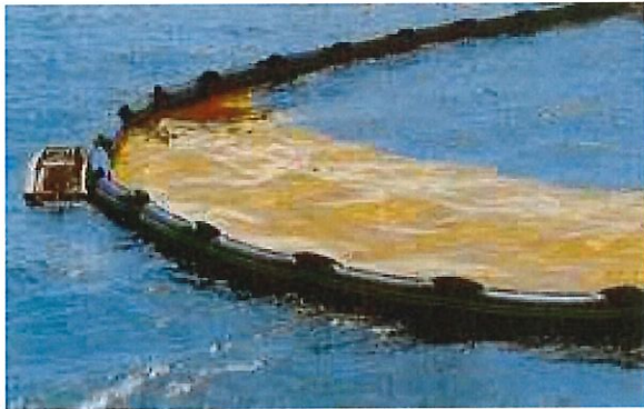
FIGURE 3-3 Containment Booming Strategies after SWA Application
